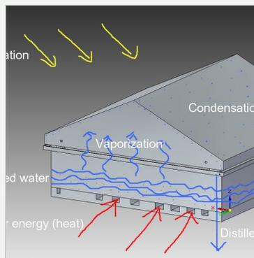
Solar water purification system with solar heating - Appropedia: The sust...
